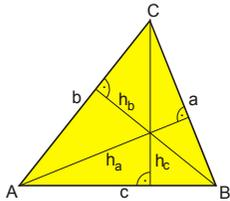
$$\begin{aligned} A_D &= \frac{1}{2} \cdot a \cdot h_a = \\ &= \frac{1}{2} \cdot b \cdot h_b = \\ &= \frac{1}{2} \cdot c \cdot h_c ; \end{aligned}$$
